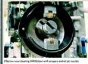
Effective rotor cleaning (MAG) clear with screens and air jet nozzles
